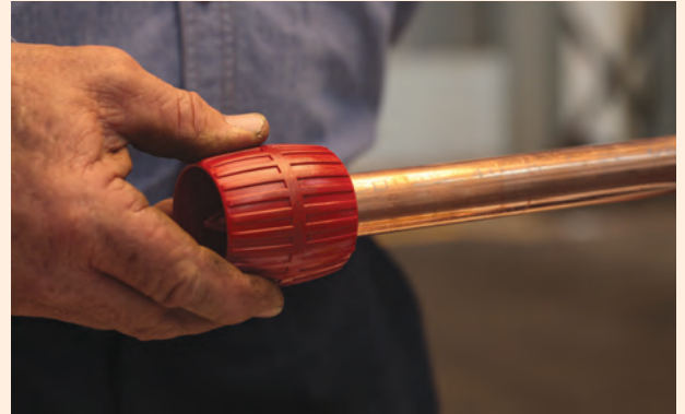
2. Deburr carefully the end of the tube on the inside to minimize turbulence and pressure loss according to AS3500 and on the outside to avoid damaging the O-ring.
