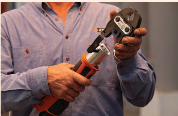
5. Select pressing jaw according to the fitting dimension and insert into the pressing machine. Arrest the locking bolts of the machine. Check the jaws are free from debris and in good working order.
