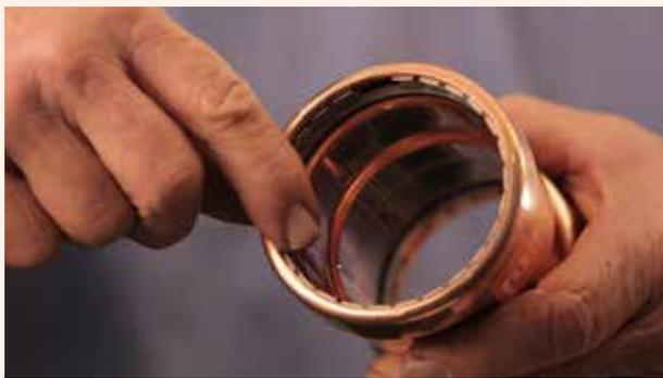
**3.** Ensure you have the correct sized fitting, check the fitting is clean and the stainless steel grip ring and O-ring are free from debris and correctly seated in the fitting.
