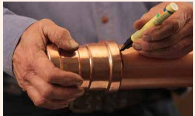
**4.** Mark the insertion depth on the tube by lining up the fitting side by side with the tube or by inserting the fitting onto the tube until it reaches the tube stop. When fitting is inserted onto the tube the outer edge of the fitting must line up with the marking. Refer to the table below for the minimum insertion depth.
