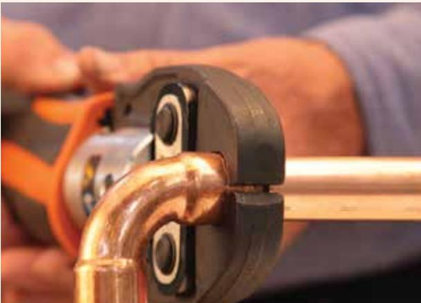
**8.** Initiate the pressing job by pressing the start button. The automatic pressing process guarantees a tight connection. The pressing process can be interrupted by pressing the emergency-stop button.
