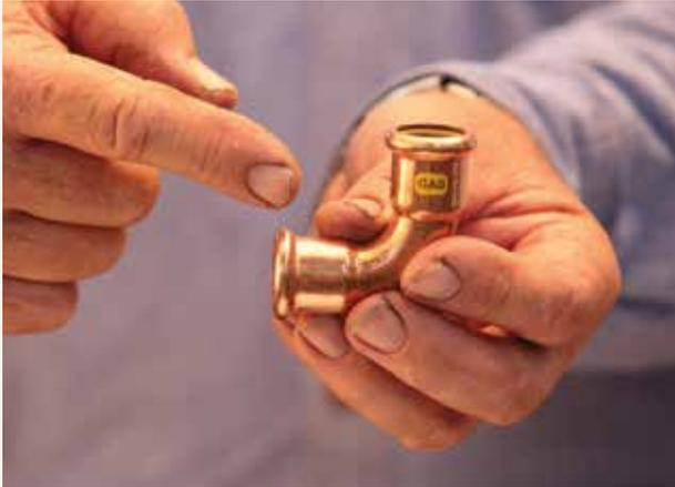
**6.** Ensure you have the correct fitting for the application (e.g. water or gas). Check the fitting is clean and the O-ring is free from debris and correctly sitting in place. Push fitting on tube all the way to the engagement marking.
