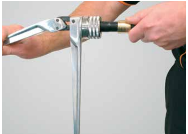
4. Open expander & rotate 30°.
