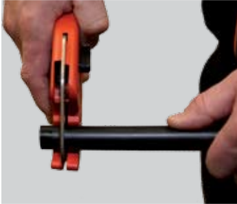
1. Cut pipe at right angle
