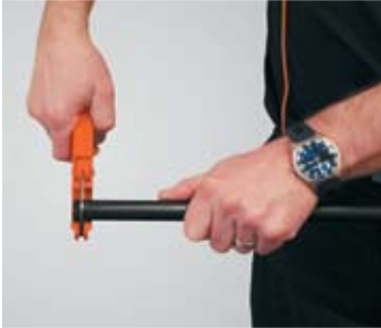
1. Cut pipe at right angle
