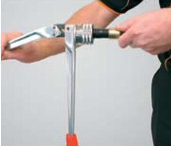
4. Open expander & rotate 30°
