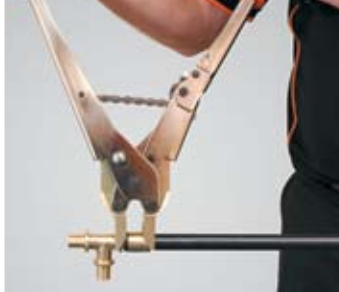
8. Press sleeve fully closed to fitting shoulder
