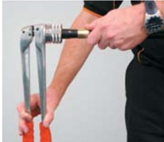
5. Expand again in new position
