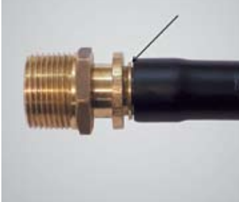
7. Ensure fitting is inserted into shoulder stop.
